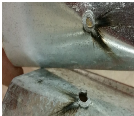
Pry test result showing weld nugget ripping free from the steel without breaking the weld.
